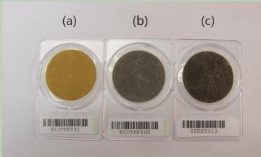
Figure 2-3. Representative Examples of Filter Samples Collected from Different Sources, including: (a) Smoldering Biomass, (b) Flaming Biomass, and (c) Diesel Exhaust. (Photo courtesy of Desert Research Institute)
